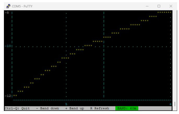
60M (BPF3) Low at -8 compared to the manual at -2. The addition of two turns on L401 should peak out this band.
