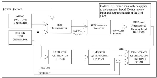
Fig. 4-8 — PTT SSB/FM RF Output Test Hook-up
