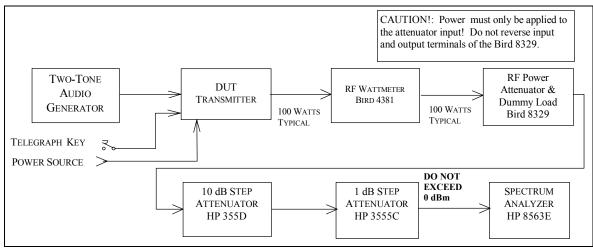
Fig. 4-5 — Two-Tone Transmit IMD Test Hook-up
