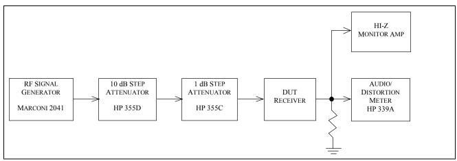
Fig. 5-11 — Audio Power Output Test Hook-up
