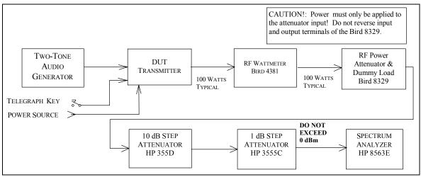
Fig. 4-6 — SSB Carrier and Unwanted Sideband Suppression Test Hook-up
