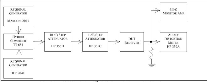
Fig. 5-8 — CW Two-Tone, 3<sup>rd</sup>-Order Dynamic Range Test Hook-up
