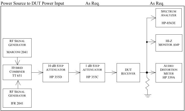
Figure 5-16 Notch Filter Test Hook-Up
