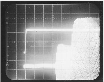
Fig. 4-9A — Oscilloscope Trace of RF Envelope
