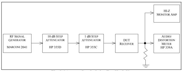
Fig. 5-6 Antenna Port Isolation Test Hook-Up
