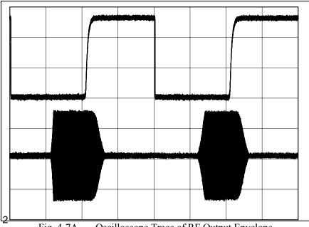
Fig. 4-7A — Oscilloscope Trace of RF Output Envelope
