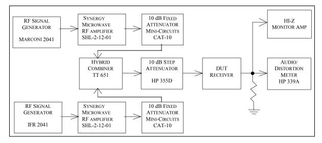
This hook-up should be used for generator levels above -14 dBm to prevent problems from test fixture IMD. The Synergy Microwave amplifiers specified are 24V "ultra-linear" units that provide approximately 25 dB of gain up to +29 dBm output for frequencies between 1 and 450 MHz.
