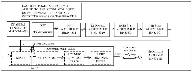
Fig. 4-11 — Composite Noise Test Hook-up
