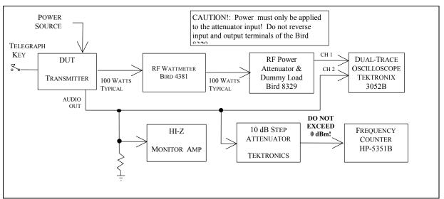
Fig. 4-10 — Keyer Speed and Sidetone Frequency Test Hook-up
