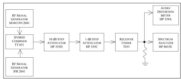
Fig. 5-7 — Blocking Dynamic Range Test Hook-up
