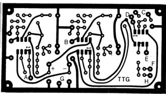
Printed-circuit board etching pattern, shown from the foil side of the board.
