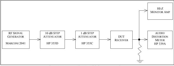
Fig. 5-2. AM Receive Sensitivity Test Hook-Up
