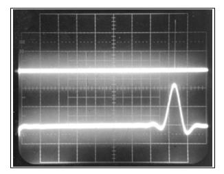
Fig 5 -- Second-phase calibration uses the BER test signal and sync pulse to produce an eye pattern. The oscilloscope is set for 10  $\mu$ sec/div. The center of the eye is adjusted to lead the sync pulse by 14  $\mu$ sec as shown.
