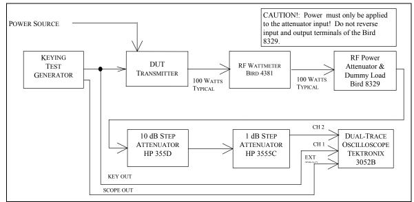
Fig. 4-7 — CW Keying Waveform Test Hook-up
