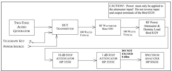
Fig. 4-4 — Spectral Purity Test Hook-up
