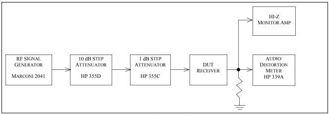
Fig. 5-13 — FM Squelch Sensitivity Test Hook-up
