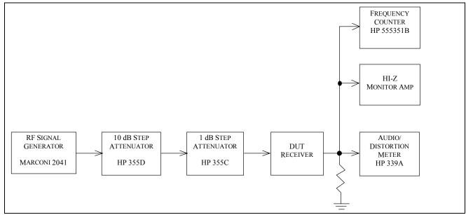
Fig. 5-12 — Audio and IF Frequency Response Test Hook-up
