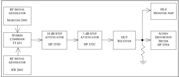
Figure 5-15 In-Band IMD Test Setup
