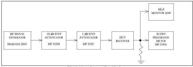
Fig. 5-14 — S-meter Test Hook-up
