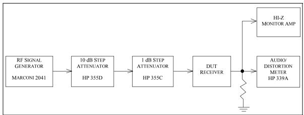
Figure 5-1 -- CW MDS Test Hook-up
