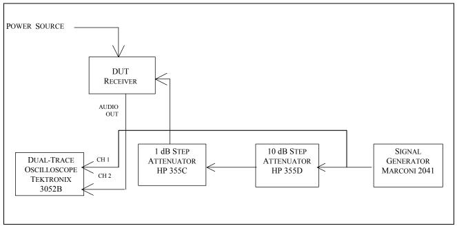
Fig. 5-16A — Notch Attack Time Test Hook-up
