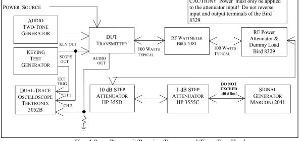
Fig. 4-9 — Transmit/Receive Turnaround Time Test Hook-up
