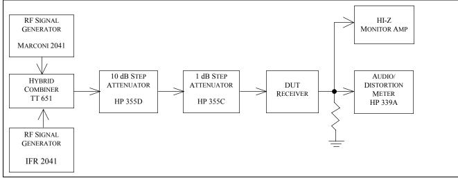
Fig. 5-9 — FM Channel Selectivity Test Hook-up
