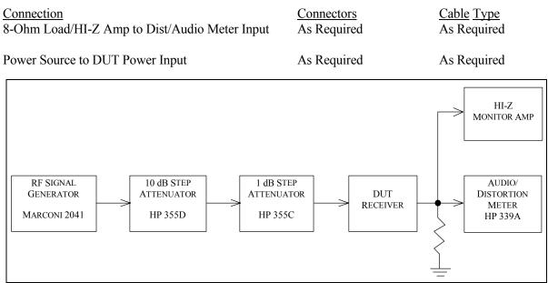
Fig. 5-4 — Receive Frequency Range Test Hook-up
