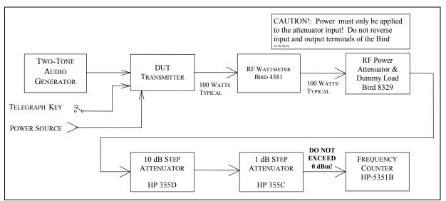
Fig. 4-3 — CW Transmit Accuracy Test Hook-up
