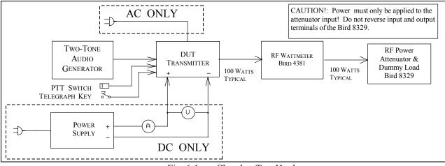
Fig. 6-1 — Chamber Test Hook-up
