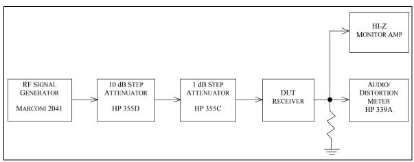
Fig. 5-3 FM SINAD and Quieting Test Hook-Up
