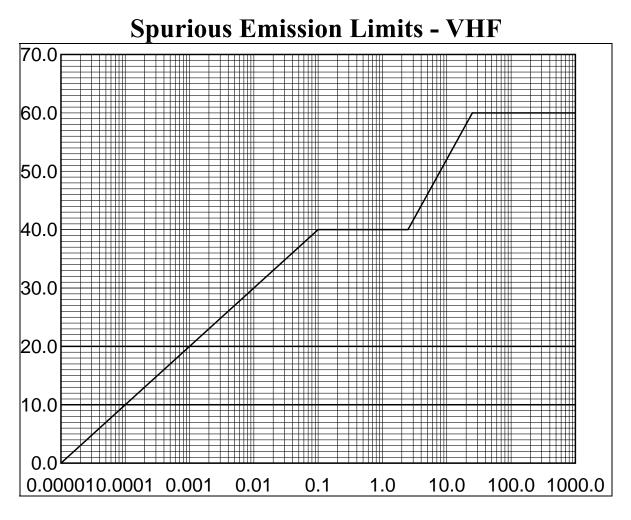
Spurious Attenuation 30-235 MHz X=Power (Watts)
