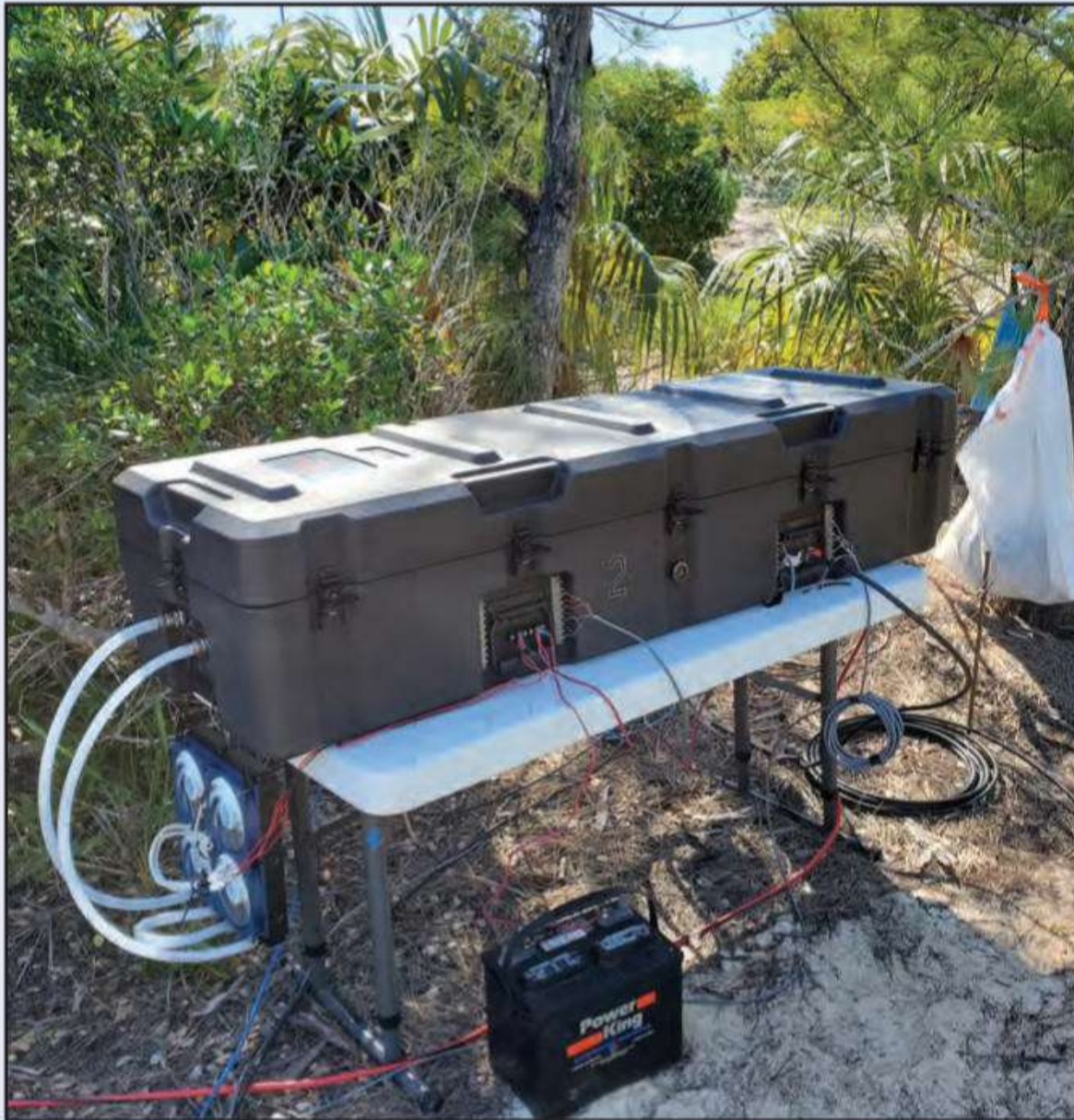
The “Radio in a Box,” or “RIB,” is a full function kilowatt station in a weather-tight box built around a Flex 6700 transceiver. It is remotely controlled from the boat and can operate unattended for days. The C6AGU group has made over 25,000 QSOs using RIBs, from an uninhabited island under pretty realistic DXpedition conditions, including during major contests. (Courtesy of C6AGU and the Northern California DX Foundation)
