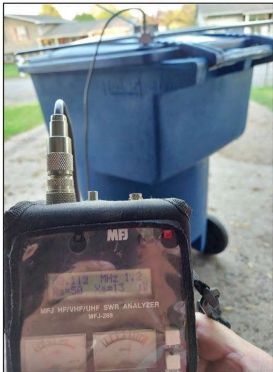
Photo I. Resetting the feed block assembly netted me a resonant frequency of 50.112 MHz and a SWR of 1.2:1!
