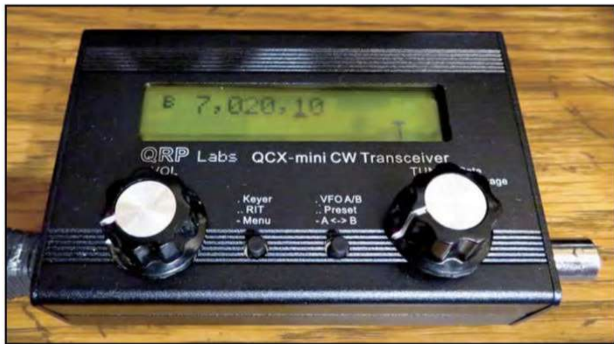
The completed QCX Mini ready to go on the air! In this mode, the copied CW can be read on the lower line of the display.
