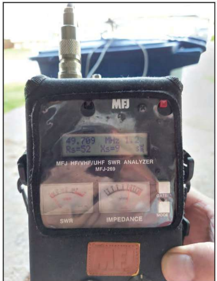
Photo H. I took the antenna outside, mounted it on top of a plastic trash can to gain more elevation and my resonant frequency shifted downward to 49.709 MHz with a SWR of 1.2:1. Height above ground does make a significant difference!
