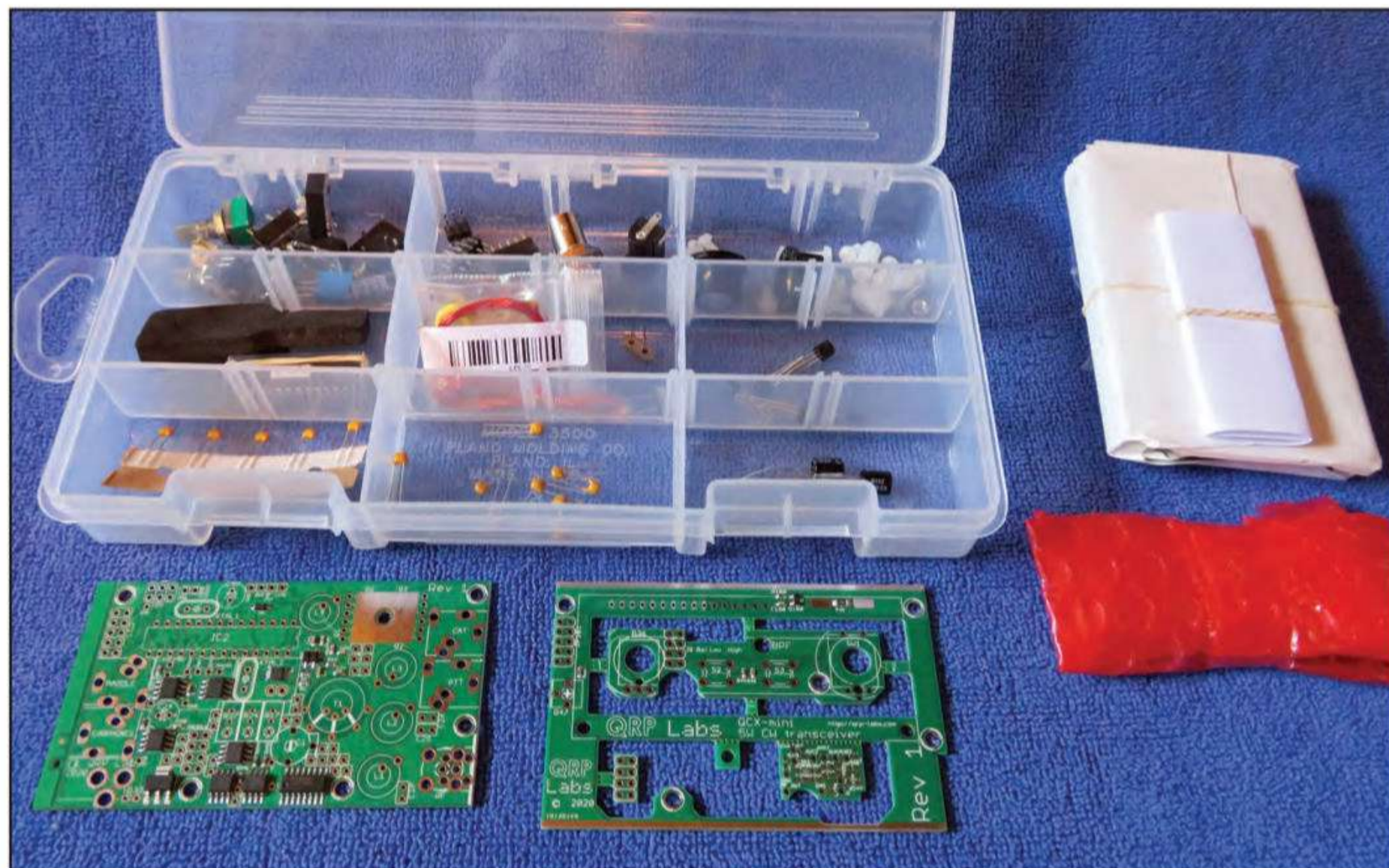
The two boards and the parts for the QCX Mini all sorted out. Notice there are no resistors!
