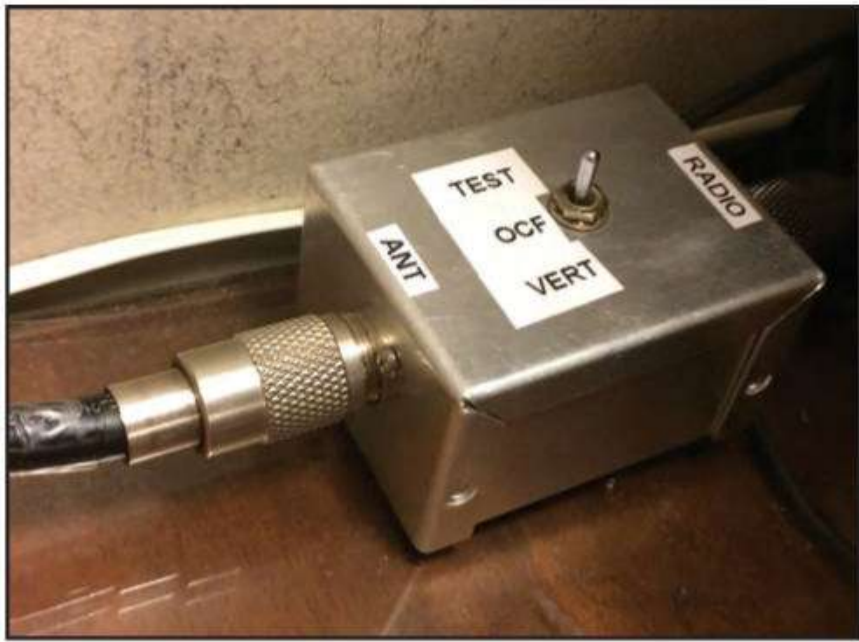
Photo A. Antenna switching controller.
