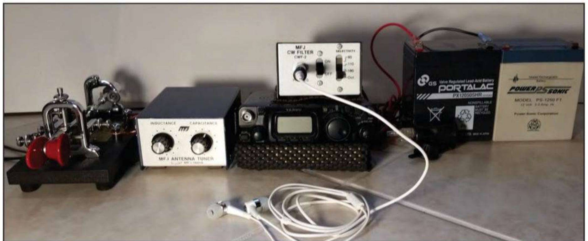
Photo C. The Baby Ruth station gear, FT-817ND, audio CW filter, tuner, bug, and batteries.
