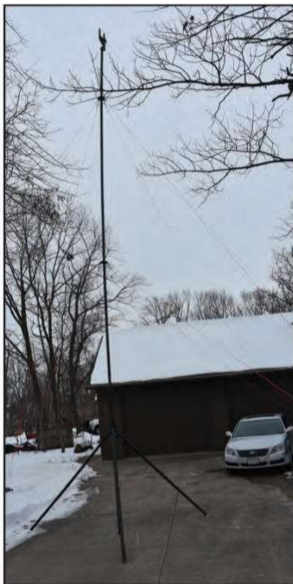
Photo C. The center-fed Zepp antenna was erected in Steve's driveway.
