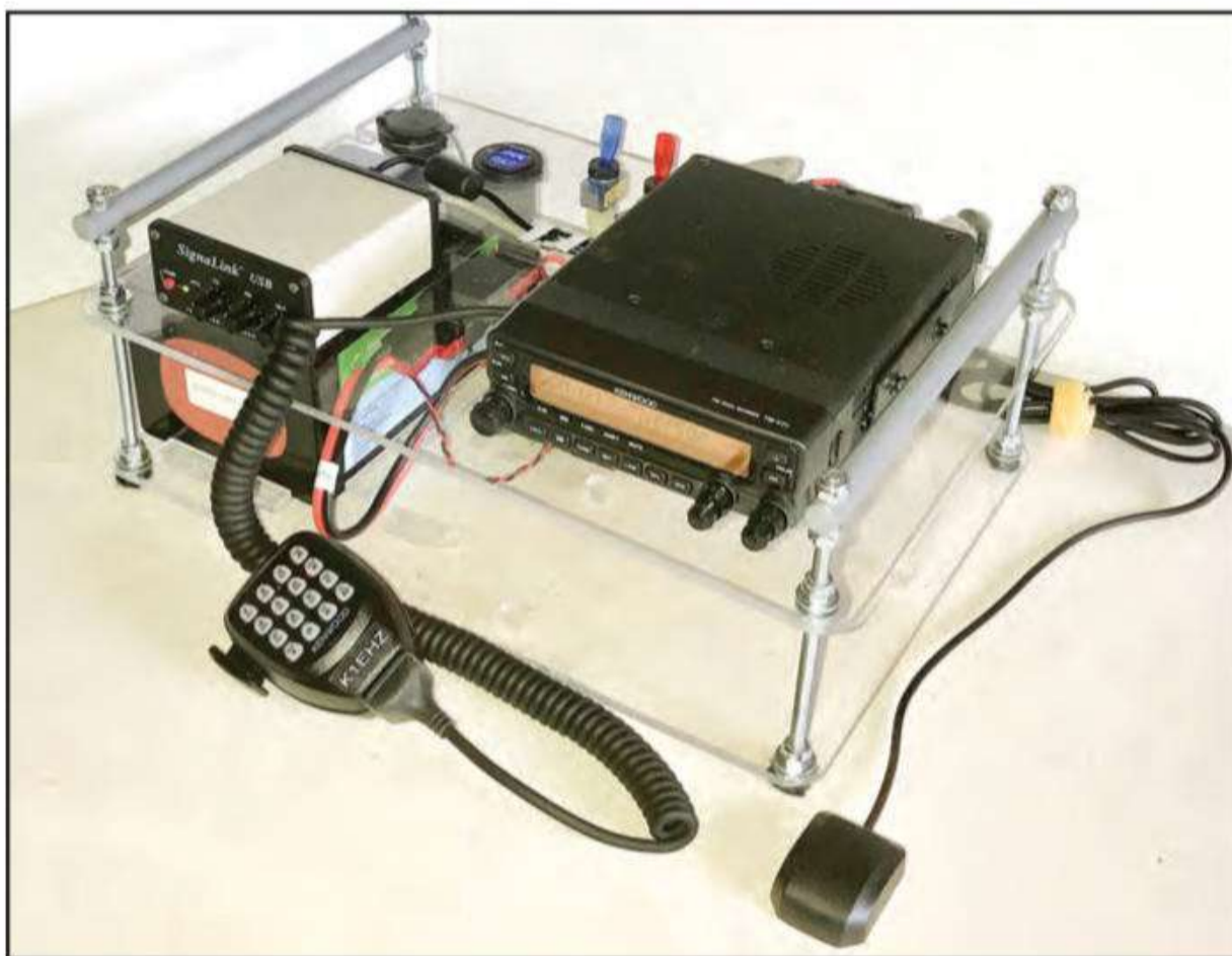
Photo C. Partially completed assembly (Note corner bolt configuration).
