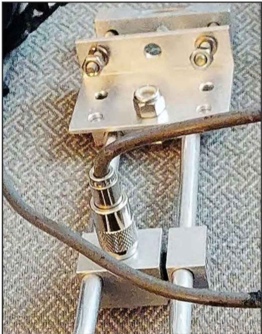
Photo D. The 6M HO loop aluminum feed block. It is easily identified because it has the UF SO-239 coax connector.
