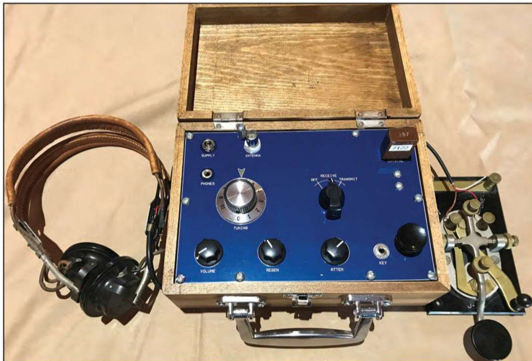
Photo B. Four State QRP Group's Bayou Jumper mounted in its optional wooden case. (Courtesy of 4SQR Group)
