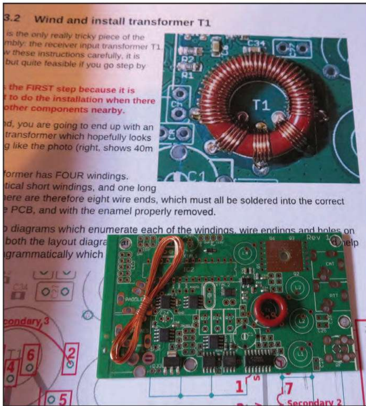
T1 is the most complex part of this kit and is done first to ensure it is done correctly. The manual is very thorough in explaining the correct way to wind and mount T1.
