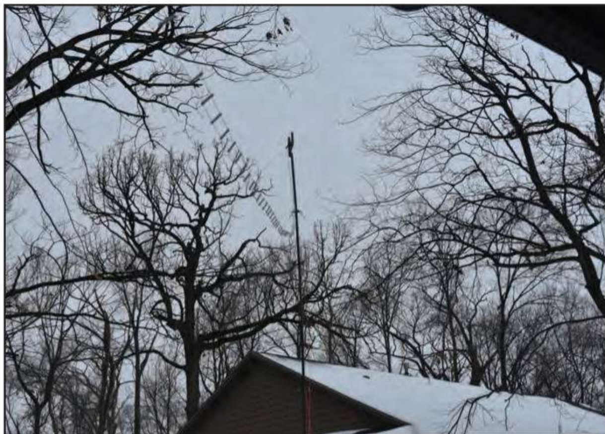
Photo D. A 450-Ohm "Ladder Line" carried the RF.
