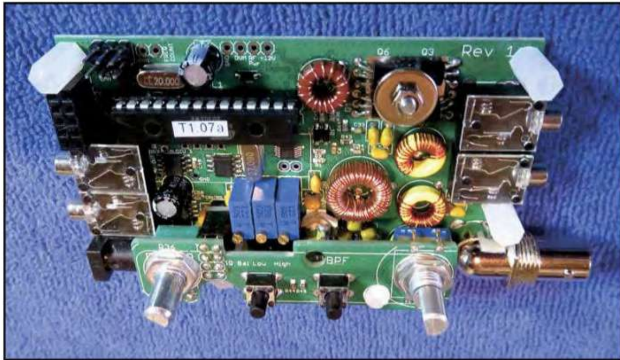
The QCX Mini without the LCD display mounted and ready for the display and testing.
