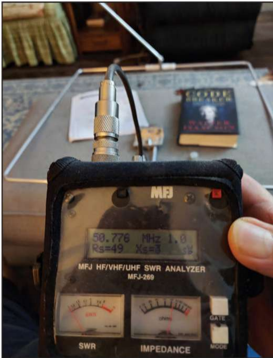
Photo G. For grins, I wanted to see just where my loop was resonating with my initial test and it was “happy” at 50.776 MHz with a SWR of 1.0:1. Better but not perfect. But wait, ground effects were at play here.
