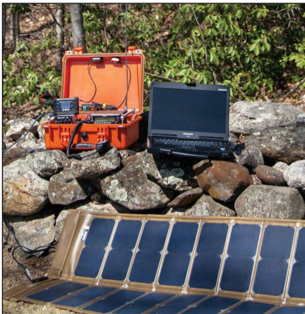
Photo A. Completed go box with solar power, laptop, and coaxial dipole antenna ready to use. (Photos by the author, except as noted)
