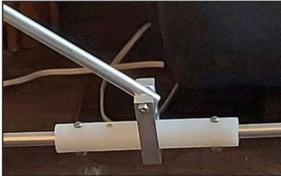
Photo C. An insulator separates each end of the 6M HO loop's tubing.
