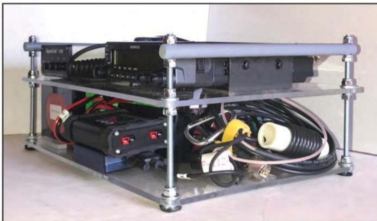
Photo G. Solar controller, battery charger, and coaxial dipole stowed between levels.
