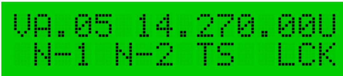
N-1, N-2 are a variable center-frequency filter, need to use with the "CW TUN" knob. N1 N2 - изменение центр при помощи CW TUNE
