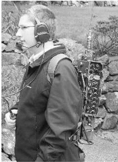
Matt Ireland, MW3YMY, is shown operating with his **Plessey RT-320**. “The radio is an RT-320 (ex British Army). The 24V battery clips onto the bottom of the rig and vertical antenna on top. The rig has an built in antenna tuner, which is very convenient. I usually trail a long radial behind me when out portable. The only downside is it is difficult to change frequency without taking the radio off your back, but I don't mind taking it off my back to tune around if necessary.”
