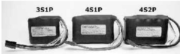
As of this writing, Buddipole is selling this type of battery. All of the A123 batteries sold by Buddipole include an integrated poly switch to prevent large amounts of over current in the event of a short circuit.
