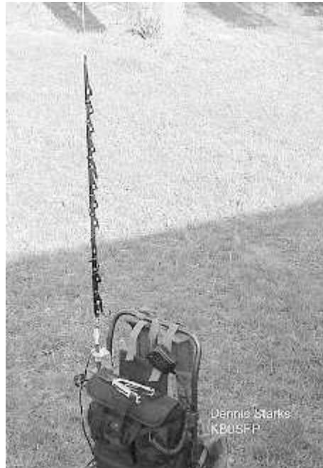
This antenna will work 40M to 2 M plus the WARC bands. It can handle twenty watts PEP and is fifty Inches tall. One additional note is that this antenna may load on 80m by using a ten foot whip. This type of loaded vertical tends to work well where low-hanging objects are in the walking path.
