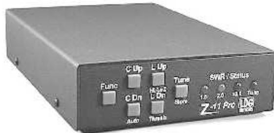
This external antenna tuner is larger in size, but can handle up to 125 watts of RF power. If you decide to use over 10W – 20W, this would make a great tuner for your HFpack. This tuner also utilizes latching-relays so it only draws 25ua of current when not in an active tuning
