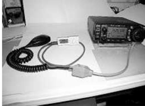
With this setup, I now just hit a button on the MP3 player and all hear my voice calling CQ over the airwaves. I works really nice and when someone answers my CQ, I just hit a button on the control head and turn off the VOX function in the radio to use the microphone.
