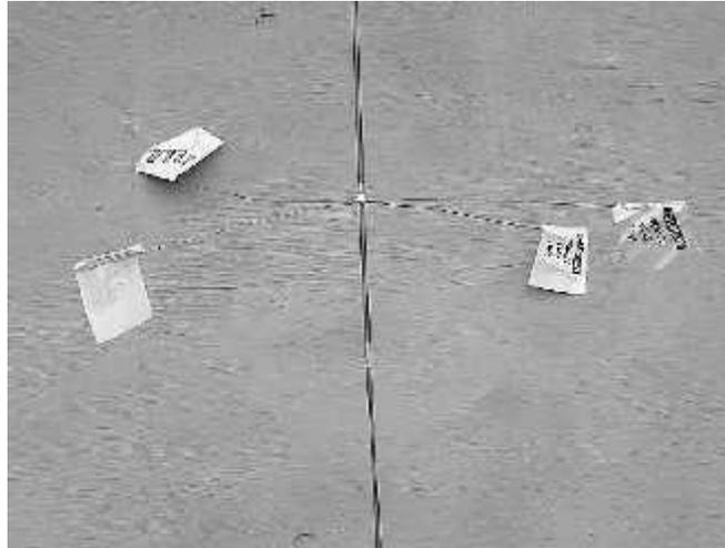
The capacity hat above was made by Paul, WORW. This top hat has four twenty-two inch spokes soldered into a small hub..<sup>9</sup> The wire for the capacity hat below was harvested from buried gas and utility line markers. Each wire weighs only two ounces. I have noticed 6 dB improvements using this top hat on lower frequencies.
