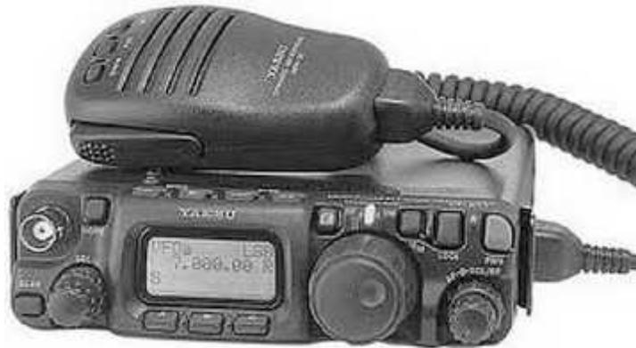
This transceiver has a receive current of only around 300ma so it won't kill your battery while out in the field. This is a one radio does it all type of rig, but with limited output power of five watts.
