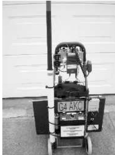
The picture below is Jose B Rivera, N2LRB and his pedestrian mobile setup that utilizes a combination of two mounting systems. He uses a hand cart mount, but also uses a frameless backpack mounted to the hand cart.
