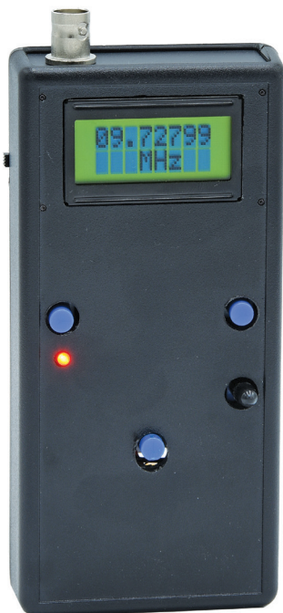
Figure 11 — The HeckKits 50 \Omega Bridge/Frequency Counter is mounted in a plastic case with a two-line by eight-character LCD.
