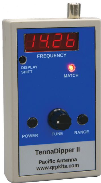
Figure 13 — The TennaDipper II in its plastic case. The controls are nicely labeled with a decal that covers the whole front panel. The builder needs to carefully cut and drill the case for the display and controls, as described in the text.
