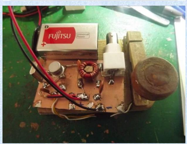
Note by SV8CYR: construct it and with the voltage 18Volt the output was 1Watt. With 9Volts 360 mW in  $50\Omega\mu$  dummy load. Transistor is 2N3866. I test and I changed trimer capacitors with permanent value C1, C2, C3. I dit not use R2, R3, D1, C6, M1.
