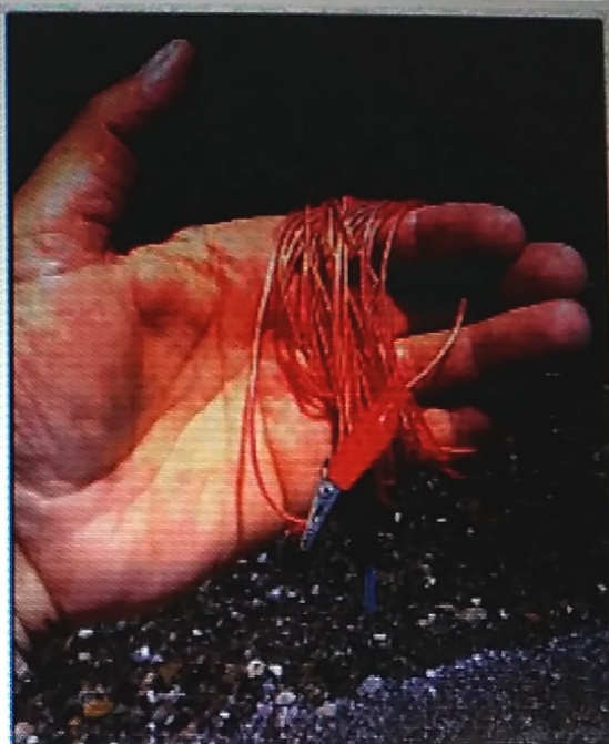
Photo E. Quarter wave wire radiator for 14 MHz with alligator clips. There were also four radials, one of which went into the lake.
